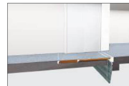
Full Closed (During Compression) During an event, the MACC system slides fully into the adjoining structure in the contraction (or compression) mode.
