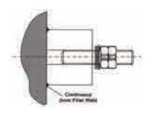
Manufactured from high quality SS316 material, it comes with SS316 stud, bolts and washers. It is commonly welded to steel vessels, tanks and structures for earthing application. Suitable for use in highly corrosive environment.
